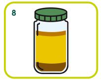
8. If the liquid is not homogeneous, try to provide a portion of each component (solids or liquids) so that the sample covers all elements.
