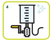
4. If you use extraction elements (suction pumps, hoses, brushes, etc.), they must be clean. If necessary, allow a sufficient amount of lubricant to carry impurities out of the circuit before collecting the sample.
