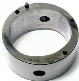
Test Denison T6H20C. Today the unique test to proclaim HF-0. It combines piston and paddle pump.
